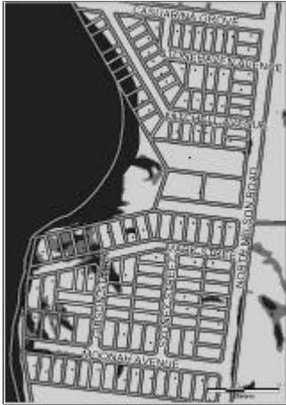
Map 1: Constraint map includes slope, stream and allotment buffers (1.5m for irrigation and 3m for trench)
